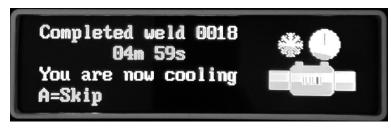
At the end of the cooling time, the fusion number is shown.
