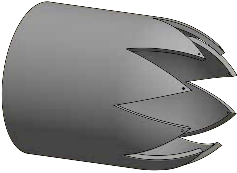
FIGURE 4-4 NOSE CONE DURING FORMING
