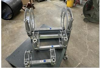
The Highland DIPS EF Straight Clamps have been designed to re-round, align and restrain 4"-12" DIPS pipes.
