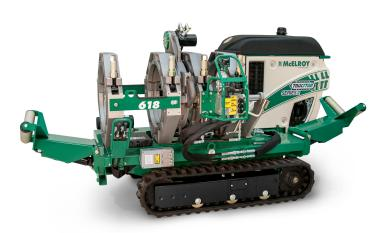
The TracStar 618 Series 2 has been completely redesigned based on feedback that came directly from the field. The new machine now shares the same vehicle with the 250 and 412 range of TracStars and is powered by a powerful diesel engine – which is especially useful on jobsites where gasoline is not permitted.
