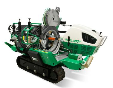
McElroy's TracStar <sup>®</sup> 500 Series 3 will butt fuse pipe sizes from 6" IPS to 20" OD (160mm – 500mm). In 1997, the TracStar 500 debuted as the world's first self-contained, self-propelled, all-terrain fusion machine. Considered the flagship McElroy fusion machine, the success of the TracStar 500 spawned the entire TracStar line of fusion equipment.
