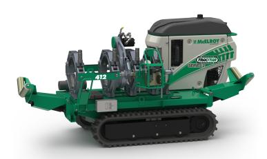
The TracStar <sup>®</sup> 412 Series 2 has been completely redesigned based on feedback that came directly from the field. The new machine now shares the same vehicle with the 250 and 618 range of TracStars and is powered by a powerful diesel engine – which is especially useful on jobsites where gasoline is not permitted.
