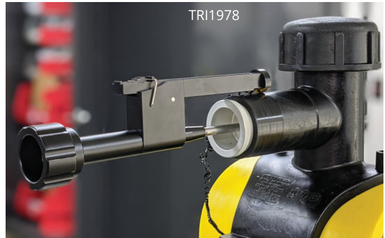
Peelers above are designed to peel a range of wall thicknesses. Peelers also available for specific wall thicknesses.
