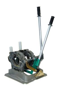
The McElroy Pit Bull 14 is a compact, lightweight, highly reliable and rugged fusion machine that fuses 1" IPS to 4" DIPS (32mm to 110mm) pipe.
