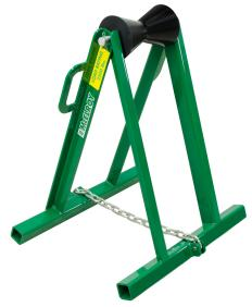
Pipe stands save wear and tear on machinery, reduce strain on operators and makes the fusion process easier. They're adjustable for uneven terrain so that the pipe is supported at the same height as the machine. By bringing the pipe in parallel to the machine it is much easier to adjust hi/low and achieve a square face-off.
