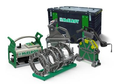
The Acrobat <sup>™</sup> 250 has a compact design for easy maneuvering in tight work spaces and is capable of fusing pipe on the ground, vertically and overhead. To further reduce its footprint, the carriage can be configured from 4 to 3 jaws without tools. A single-size insert design can accommodate a variety of pipe sizes, and its narrow jaws allow fusions to most flanges and fittings.
