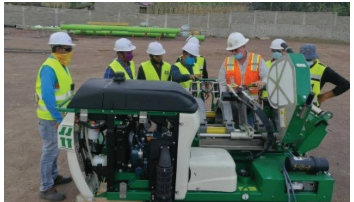
ISCO operator conducting onsite HDPE fusion training for installation personnel on McElroy 2065 fusion machine (above), and McElroy Automated 412 fusion machine (below).
