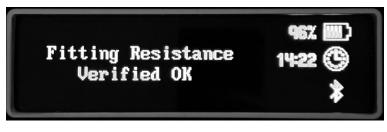
Scan the traceability code on the fitting or press the A key to move on.
