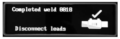
Disconnect the output leads from the fitting to reset the machine.
