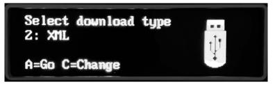
Insert a USB memory drive into the USB port on the machine. You may have to remove the barcode dongle first.
