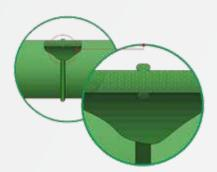
Similar to HDPE, Aquatherm is a monolithic fusible plastic that is fused together through a combination of heat and pressure. This process takes just minutes – not hours like other materials. Installed correctly, it will remain leak-free for decades.
