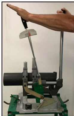
Torque Wrench Adapter (left) Part number: 410802
