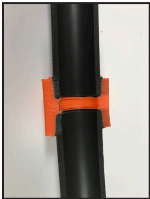
Inside cross section of socket fusion.
