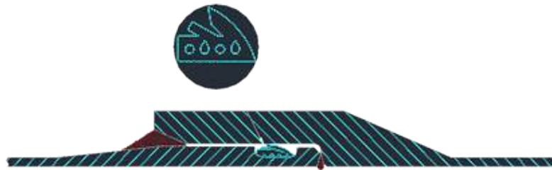
Spirolite Thermal Welded Bell and Spigot Joint
