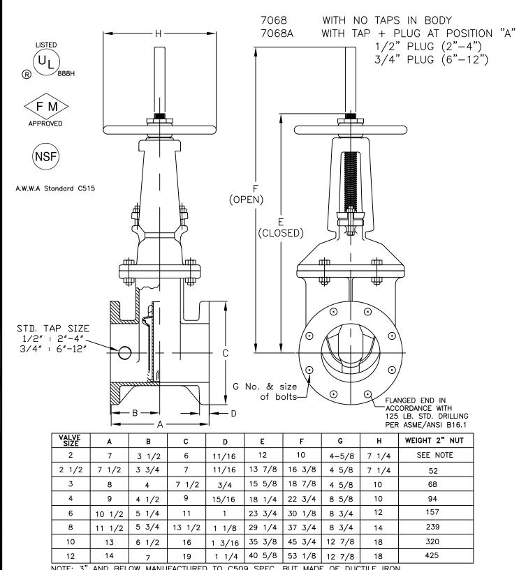
NOTE: 3" AND BELOW MANUFACTURED TO C509 SPEC, BUT MADE OF DUCTILE IRON NOTE: 2" CONSULT FACTORY FOR AVAILABILITY --- AWAITING UL APPROVAL TURNS TO OPEN: 7 3/4(2"), 8(2 1/2"), 10(3"), 13 1/2(4"), 19 1/2(6"), 25 1/2(8"), 31 1/2(10"), 37 3/4(12")
